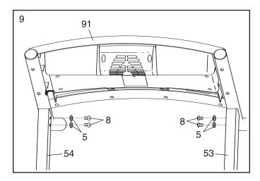
10. Tighten two M8 x 15mm Bolts (8) with two M8 Star Washers (5) into the Uprights (53, 54).
